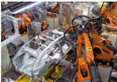
We develop methods to reduce energy consumption on robotic production lines welding at Skoda Auto that contain up to 700 robots
